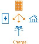
As your SunPower Equinox® system produces energy, it sends what you're not using to SunVault® storage and/or sells it back to the grid.
